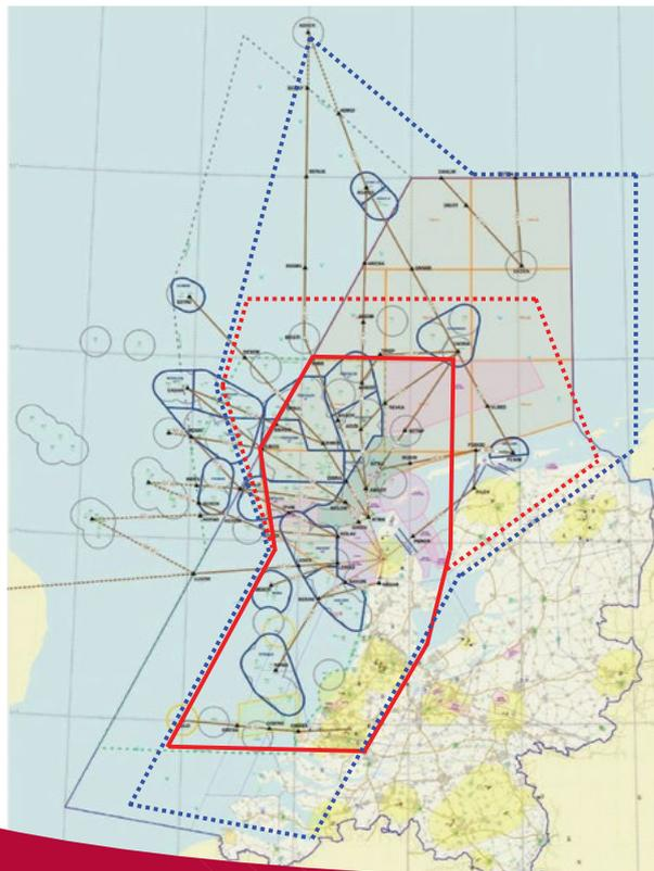
The area is covered from 1,500 ft till 45,000 ft except the Main Helicopter routes and Helicopter protection zone's which are covered from 500 ft. ADS-B covers the area from 100 ft till 45,000 ft. The system has already passed a one year long successful trial and was officially accepted as operational.
