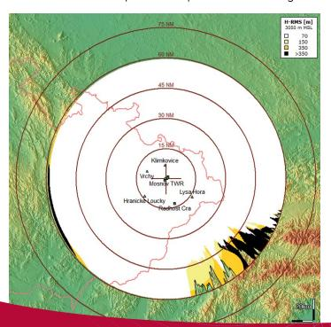
The picture shows the actual coverage and accuracy after the last extension at the flight level 100 (that means sea level 3050 metres). The coverage extends 80 NM from the Ostrava airport all the way down to the airport surface.
