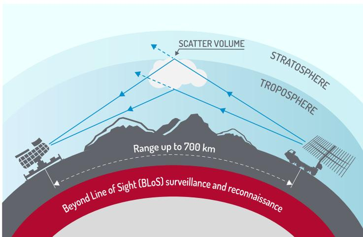
PLESS makes use of the troposphere reflectivity properties, which enables the detection of targets at a distance even beyond the radio horizon.
