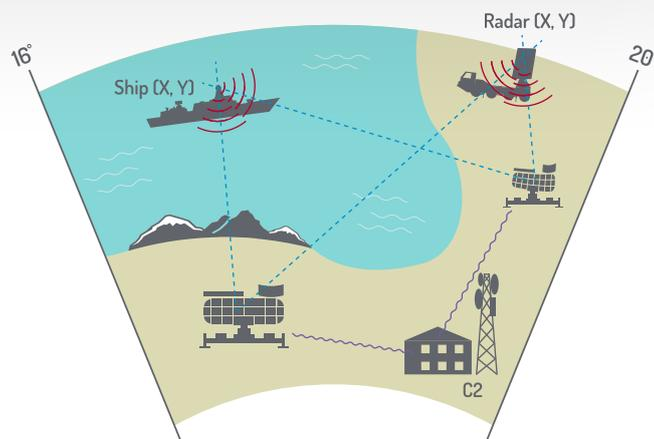
The principle of operation is the same as for any usual DF, where the sensor is measuring the Angle of Arrival (AoA) of the signal. For the 2D location of the target, at least 2 separate sensors are needed. The target position is estimated by the triangulation principle.
