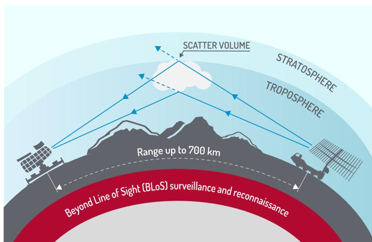
PLESS makes use of the troposphere reflectivity properties, which enables the detection of targets at a distance even beyond the radio horizon.
