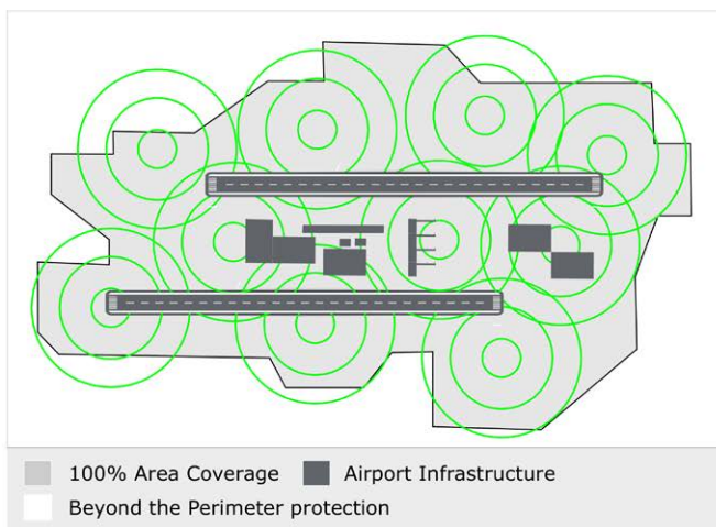
4 EHF radar network. The number of radars and their deployment depend on the geographical conditions of the controlled airport area.
