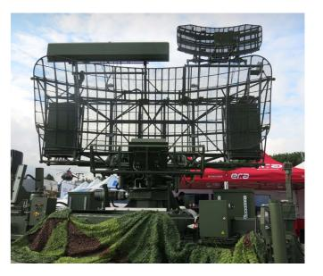
PLESS is a passive Over The Horizon (OTH) Direction Finding (DF) system developed by ERA. This direction finding system can detect, locate, identify and track air, land and naval targets with a focus on slow-moving or stationary platforms. The system processes signals from radars, jammers and datalinks emitting in a frequency band from 100 MHz to 18 GHz.
