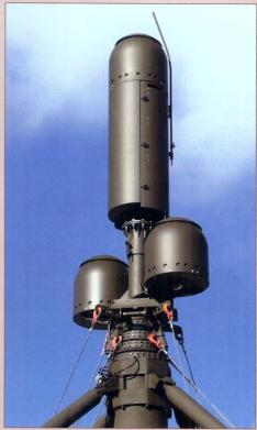
ERA has created the ultimate, world-leading and advanced Passive ESM Tracker (PET) VERA. Its 5<sup>th</sup> generation VERA-NG utilizes MLAT techniques to locate and track targets by multilateration on various electronic emissions in a broadband range. The passive technology utilized by ERA allows for a virtually undetectable operation, it emits zero electromagnetic energy making it invisible to anti-radar missile systems. It sees without being seen!
