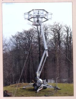
The demonstrator of passive surveillance systems known as Silent Guard implemented ERA's PCL and PET (VERA-NG) systems for the 1st time ever. The PCL (or else MSPSR in Eurocontrol terminology) demonstrator has been developed as an FM based multistatic
