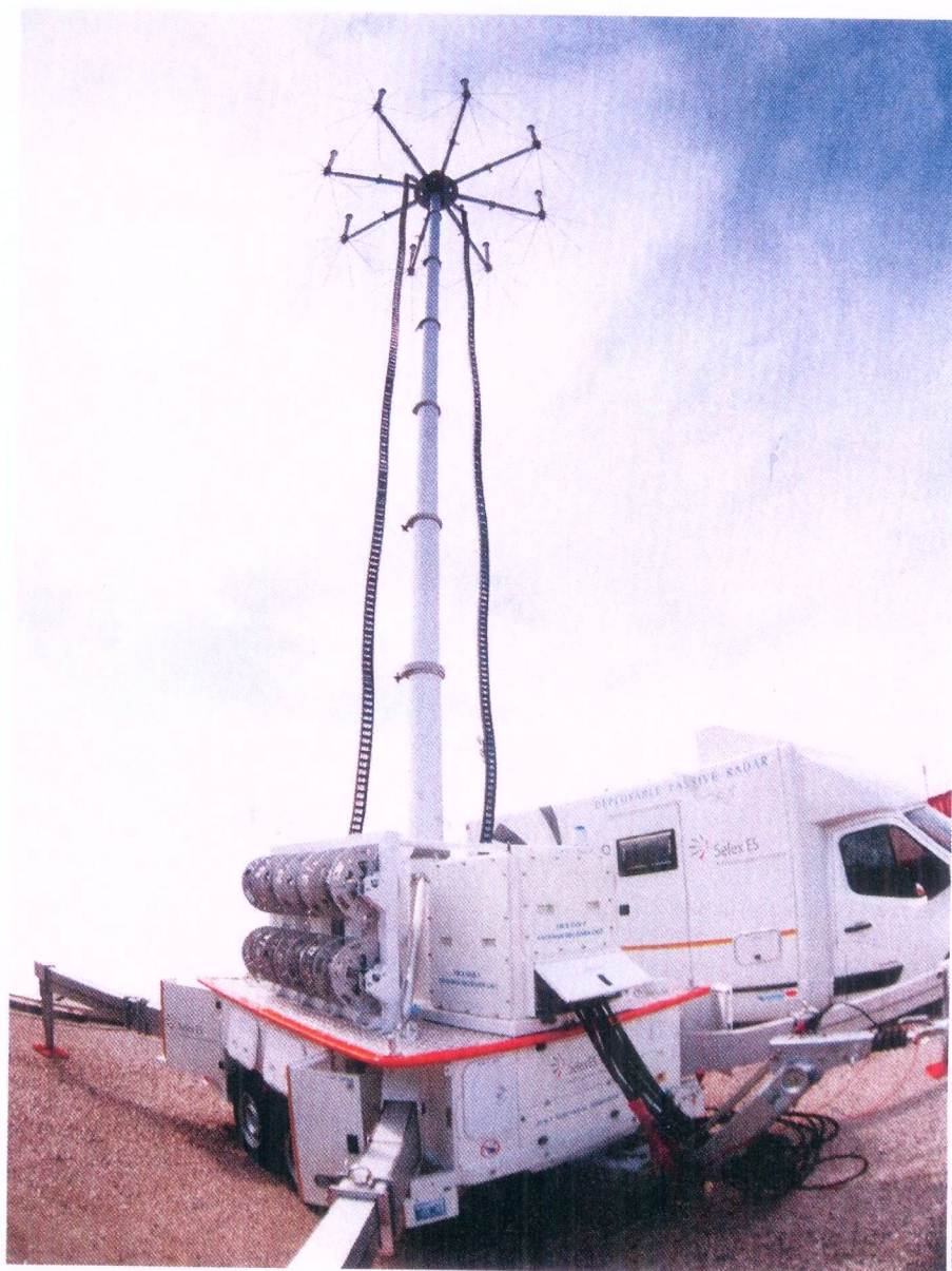
Selex's AULOS passive radar is available in two versions: one that provides speed and range information, with the second providing altitude information for aerial targets. AULOS performs these functions through the detection of FM radio signals.
